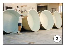
We manufacture one piece round tanks up to 8' 6" in diameter. Tanks over 8' 6" diameter are usually produced in two or more sections in order to be road legal, which saves on freight as it does not require a wide load permit. Round tanks are available with a flat or a tapered bottom. Most models over 4' deep require the installation of top jump rings to achieve the added height and require assembly.
