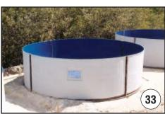
Our round multi sectional panel tanks are available in 20' 6", 25' 6" and 30' 6" diameters in many heights up to 8'. The bottom of these tanks can be assembled flat or tapered with the addition of an 8' round 5 degree donut shaped center circle. Also included is a center sump available in a round or pyramid style. All multi sectional tanks include the necessary hardware (resin, fiberglass tape, stainless steel nuts & bolts, caulking, gel-coat, etc.), and directions for assembly.
