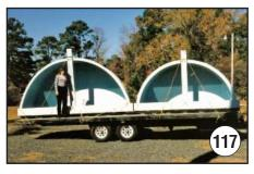
We have six sizes of large, ½ round grotto aquariums. This grotto shape is ideal for fish display, because it causes the fish to stay in the front center of the tank for better viewing. These tanks are manufactured by using half of our 10' 6", 12' 6" or 15" 6" two piece round molds. We glass on a fiberglass face panel and then install a sheet of acrylic from the inside. These tanks are available in 4' or 6' depth.
